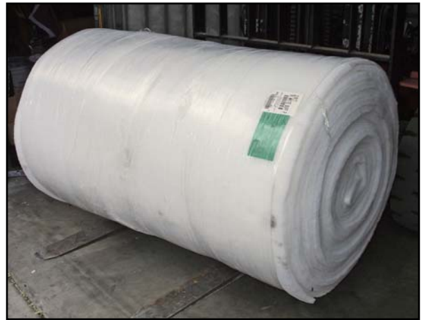
Exhaust filter media; paint booth filters
