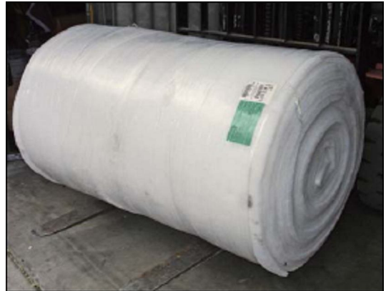
Exhaust filter media; paint booth filters
