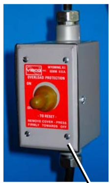
Remote Power Switch (Variable Speed Controller Optional)
